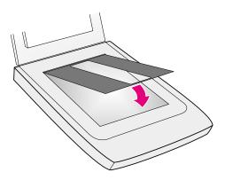
3 Slide the strip of negatives into the negative holder. If the negative strip curves, the curve should be facing out toward you.
